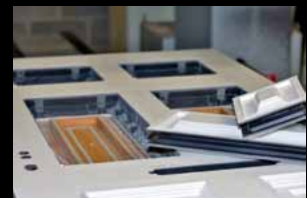
Door after routing operation
